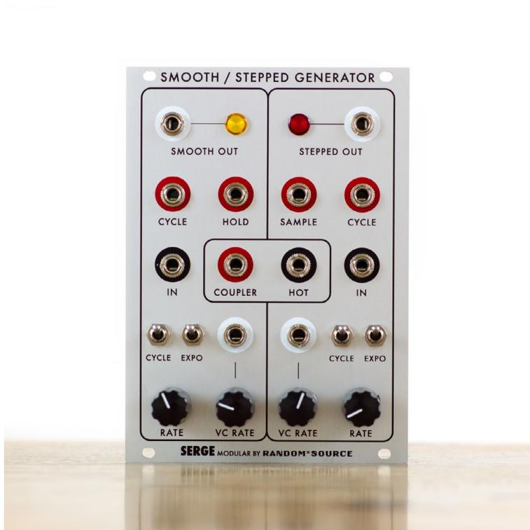
The Smooth section will place a positive and negative slew on input voltage transitions for lag effects, voltage controlled portamento and for low frequency filter applications." In Cycle-mode (cycle jack patched to the input), the Smooth side "will oscillate yielding a voltage controlled triangle wave LFO. A high level into the HOLD input will enable the Smooth Function to be used as a track-and-hold circuit with voltage controlled slew rate.
