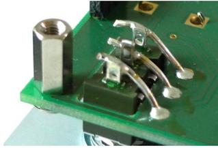
12. Solder the banana jacks in. You can either solder them directly to the surrounding vias (the ring around) or - which makes removing easier should you ever need to do that - by inserting a stiff (bare) wire into the little hole (via) and solder that wire to the top of the banana jack:
