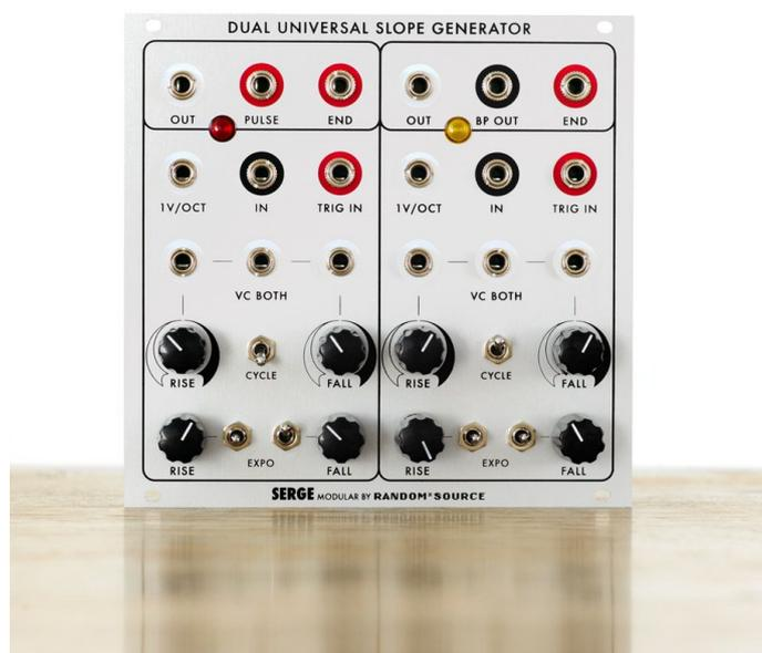
The Serge Dual Universal Slope Generator DSG is one of the most versatile modules in the Serge system. The DSG mk2 by Random\*Source is a licensed and authorized adaption of the original Serge design. Like the first R\*S version of the DSG it offers **independent VC control over RISE and FALL**.
