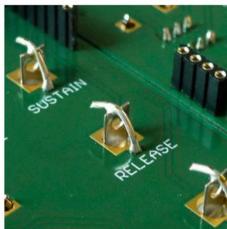
13. Attach any screws / spacers if desired and mount the main pcb onto the component pcb.
