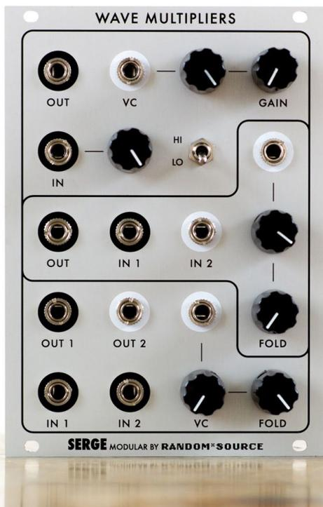
The **middle section** generates a sweep of the odd harmonics (1, 3, 5, 7, 9, 11 and 13th) when a sine wave is applied to its input and the FOLD knob is turned up or a control voltage is swept from low to high. This effect is similar to overblowing a wind pipe closed at one end. A second input is included to allow two signals to be mixed before processing. This module can be used to explore timbral areas beyond the range of ring modulation.
