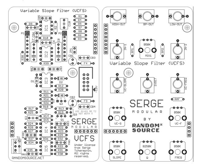
The Serge Variable Slope Filter consists of a main pcb and a matching component pcb serving as an interface to the front panel:
