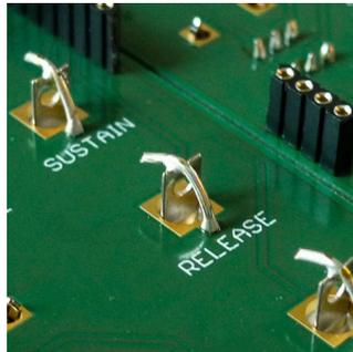
13. Solder the wires for the switch onto the corresponding switch terminals.
