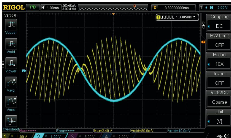
(B) Turn the MODE knob to center position (AM). When feeding a saw wave into the CARRIER, you should be able to get a beautiful amplitude modulated OUTPUT like this:
