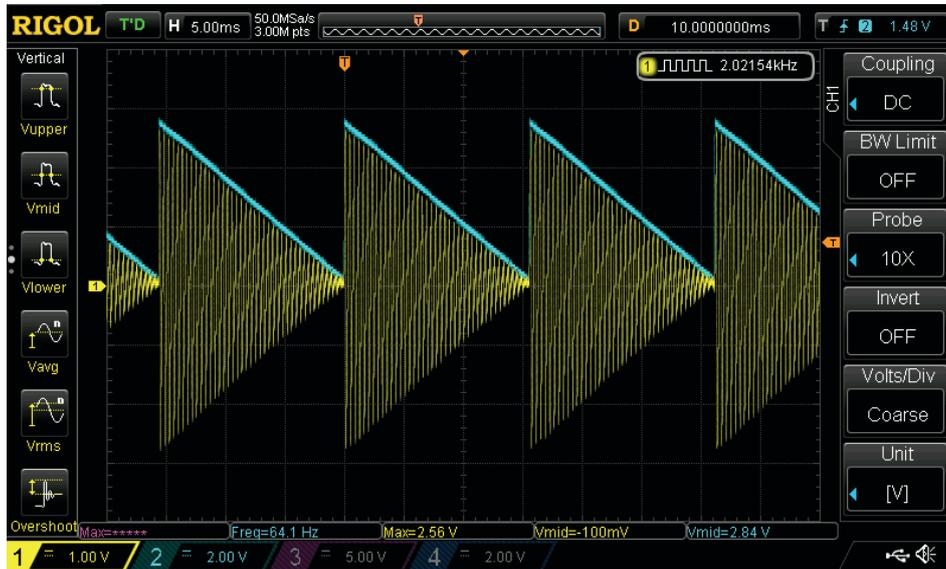
Beware that the signal and carrier level going in will affect the symmetry - a DSG mk2 will show an increase of amplitude when either Rise or Fall is very steep (towards the ends of the knob ranges) - the module is designed to work with 0-5V / 5V pp levels going in (i.e. standard Serge signal levels) - thanks to the input attenuators any “hotter” signal levels should be no problem, however, for calibration it is recommended to use a 5V signal and have the attenuators opened all the way.
