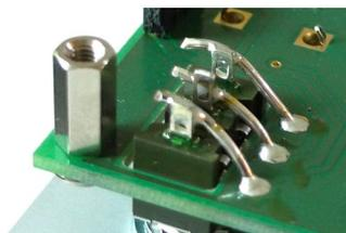
10. Solder the banana jacks in. You can either solder them directly to the surrounding vias (rings around) or - which makes removing easier should you ever need to do that - by inserting a stiff (bare) wire into the little hole (via) and solder that wire to the top of the banana jack:
