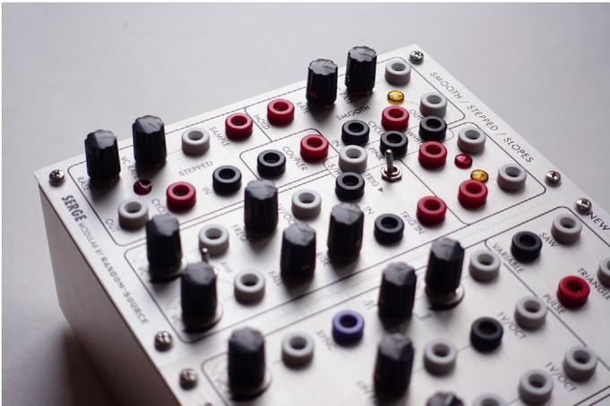
“Carnivore” combines three key Serge modules in only 4 inches: a Serge Smooth & Stepped Generator (SSG), a Serge Noise Source and a Dual Universal Slope Generator mk2 in a slim, oscillator-oriented version covering the functionality of what’s sometimes called “VC TIMEGEN” oscillator (and more).
