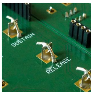
11. Solder the through-hole parts onto the main board.
