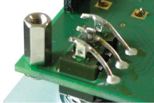
8. Solder the banana jacks in. You can either solder them directly to the surrounding vias (rings around) or - which makes removing easier should you ever need to do that - by inserting a stiff (bare) wire into the little hole (via) and solder that wire to the top of the banana jack:
